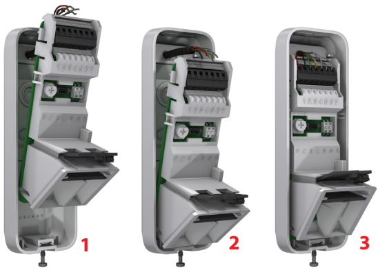
Figure 5 – Attaching the Main Unit
