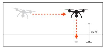
**B)** When flying lower than 33 feet (10 meters) the TYPHOON will climb to 33 feet (10 meters) while flying back to the home point, or active home position, then descend vertically until it lands.
