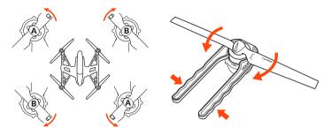
Each motor and propeller are marked with an 'A' or 'B' to ensure easy installation in the correct positions (for example: install propellers marked with 'A' on motors marked with 'A').
