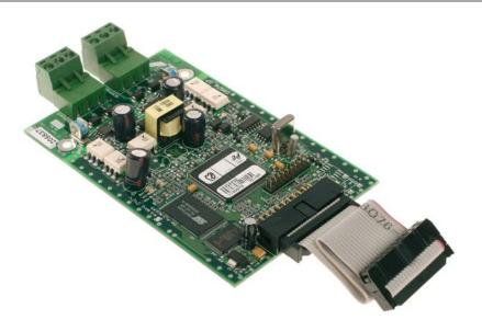
The VESDAnet<sup>™</sup> Interface Card (VN Card) is a simple interface card for the range of Xtralis VESDA VLF smoke detectors. The VN Card provides seamless VESDAnet communication from the detector to other VESDAnet devices, including configuration and monitoring tools.
