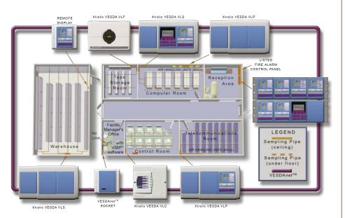
Having all Xtralis VESDA smoke detectors on a VESDAnet loop allows you to configure and interrogate each detector from a central location, in this case the Facility Manager's office.
