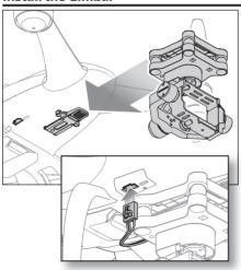
Install the gimbal by lining up the mounting rails of the gimbal and the mounting plate and pushing towards the rear of the plate as shown at left until it locks into place.
