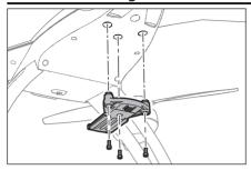
The GB203 gimbal is compatible with 350 QX3 and Chroma $^{\text{\tiny M}}$  quadcopters. Install the appropriate mounting plate using the 3 included M2.5 x 10 screws. **Do not overtighten.**
