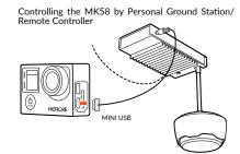
STEP 1. Plug the MINI USB connector into USB interface of GoPro Camera
