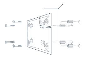
PICTURE 2. SmartBracket wall installation scheme
