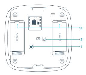
PICTURE 3. Battery compartment
