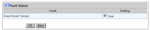
The fault events that exist in the alarm system is displayed under this section. When fault event exists in system, the control panel Fault LED will light up to indicate fault status under Disarm or Home Arm mode (The Fault LED will not light up under Arm mode).
