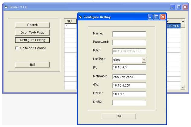
The LanType is default to **DHCP** and does not require manual input of IP/Netmask/Gateawy/DNS setting. If you wish to configure these setting manually, change LanType to **Static**.
