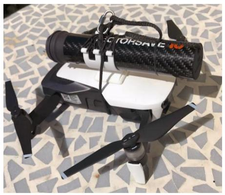
Place the clip on the center of the frame
