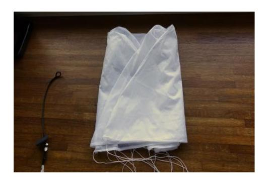
Lines should be positioned to loop inside along the centerline while the shock cord is left outside. [p]
