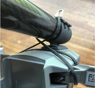
Make turns under arms and then return up by crossing the lines. Then mount the shackle under a rubber band.
