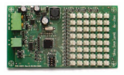
The SmartMimic board allows you to create a synoptic panel by means of an overlay which attaches to the panel front. This is done by perforating the overlay in the positions which represent the zones and wiring up the corresponding LEDs by means of the wires supplied with the board. The board connects to the RS485 BUS of the SmartLoop control panel and accepts 48 LED connections.
