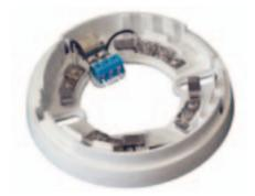
Relay base (mod. EB0020) with programmable relay base (contact NC and NO) controlled directly by the detector microprocessor. If combined with Enea series detectors, the activation logic can be defined independently for each relay base through the SmartLeague programming software. The EB0020 base can be used to connect IRIS detectors to an intrusion control panel.
