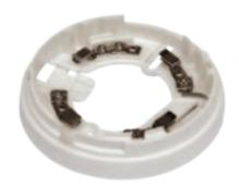
Standard base (mod. EB0010) for the electrical connections of IRIS and ENEA detectors on closed-loop lines (max. 240 ENEA detectors per line) or conventional lines (max. 32 IRIS detectors). Complete with power supply and alarm contacts. Equipped with short-circuit plate which ensures continuity in the event of removal of the detector from the line.
